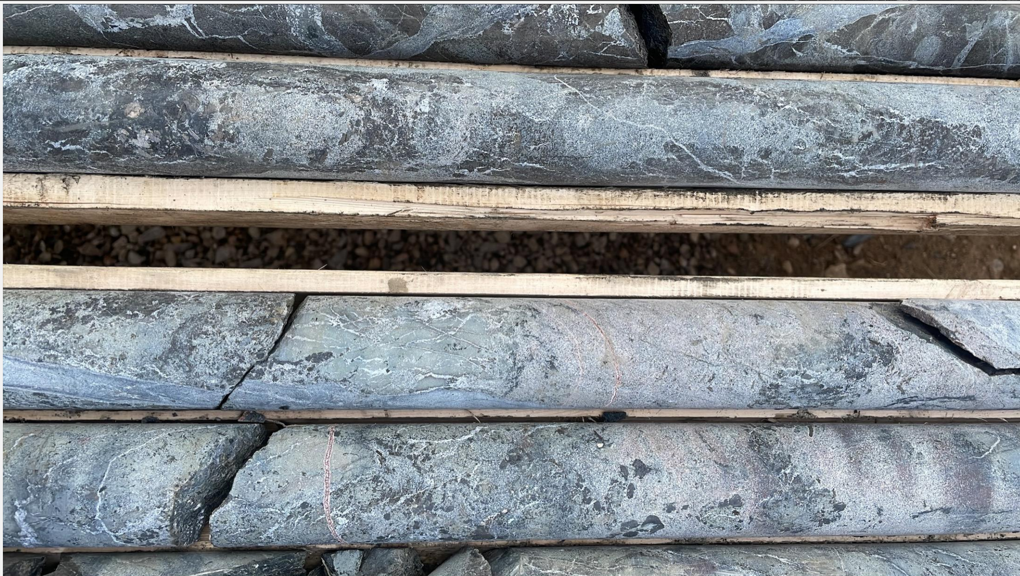
Photograph of drill core with 2.2% TREO and 19% P205 at 219m in hole HK22-013. Rare earth element mineralization is amongst a myriad of carbonatite dykes (phoscorite and sovite) which themselves are cut by fluorite-rich carbonate veins. Protolith alkaline igneous rocks are completely replaced by a potassic alteration assemblage (fenite) dominated by hydrothermal biotite.
