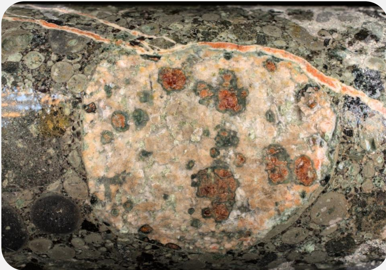
Garnet-bearing eclogite xenolith with kelephyte rims in packed, accretionary pyroclastic kimberlite diatreme breccia, Hole NW22-001
