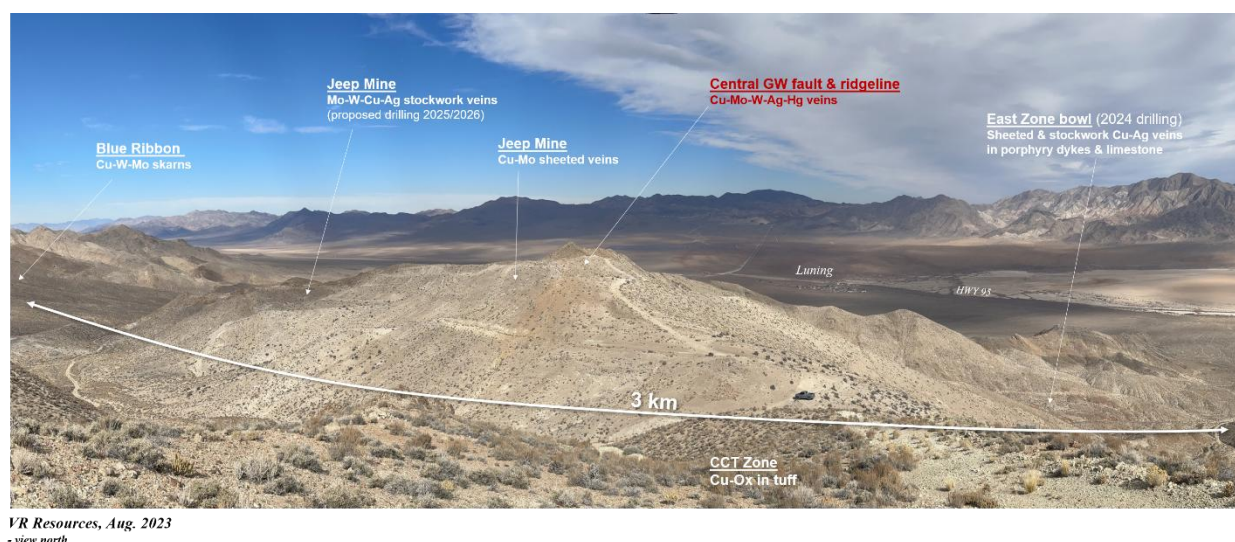
Figure 4. Field panorama photo, VR Resources, August, 2023, view north, showing the expanse of the Cretaceous New Boston polymetallic tungsten-moly-copper-silver porphyry-skarn system in west-central Nevada. It is hosted in Triassic limestone, with sheeted quartz monzonite dykes and sheeted and stockwork veins exposed on surface over a strike length of 3 - 4 km east-west.
