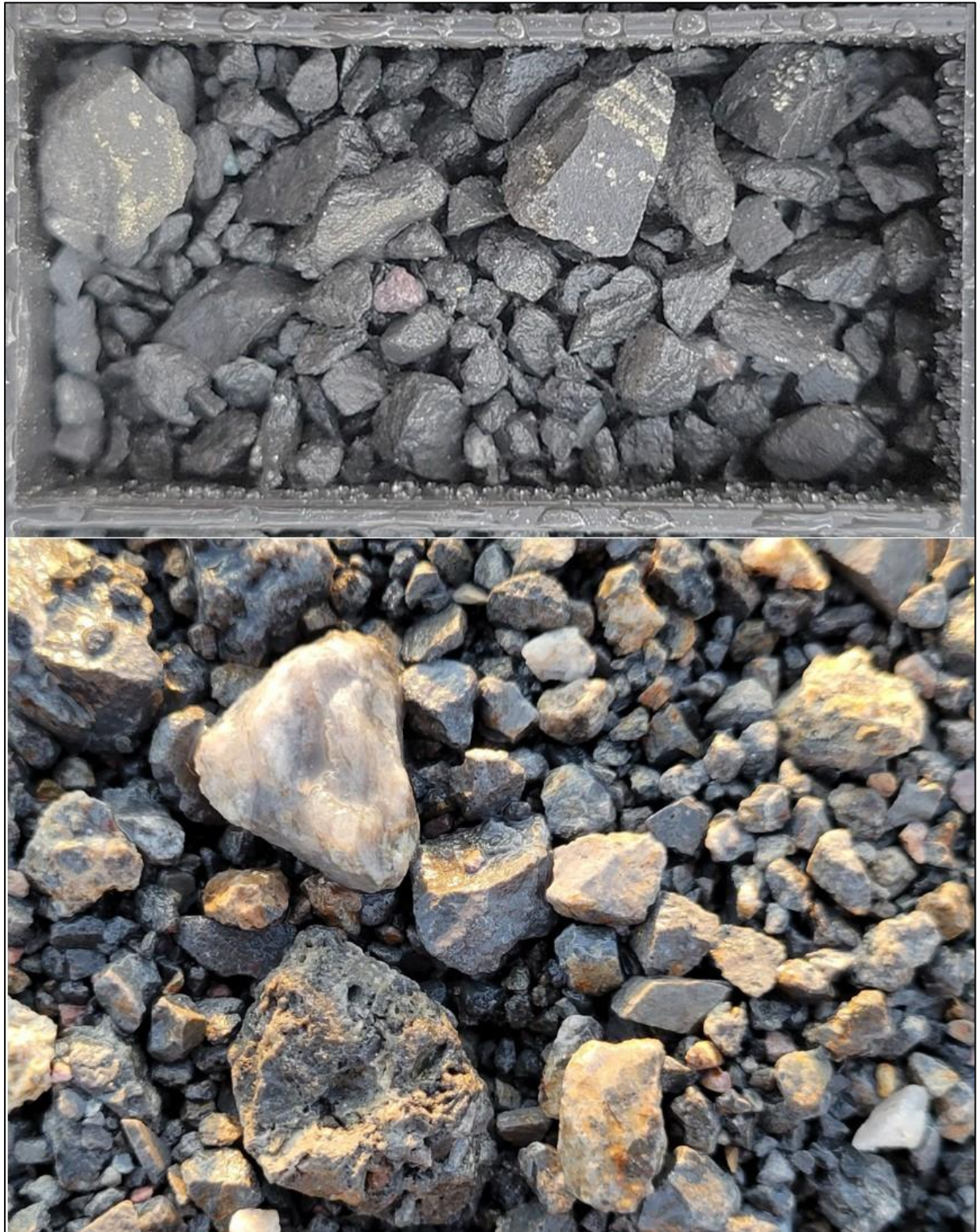
Photo 2. Drill chips from the Kawich IP anomaly. Upper photo: sulfide seams and disseminated blebs associated with bedding parallel replacement of completely decalcified and silicified, black lime mudstone at 160 m hole depth in Hole RV21-007. Lower photo: oxidized sulfide grains in leached stockwork quartz veins with secondary calcite in zones of hydrothermally brecciated, altered (dolomitized and silicified) black lime mudstone at 285 m in Hole RV21-008.
