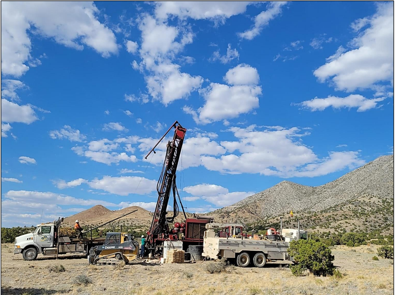
Photo 1. The truck-mounted RC drill rig set up on drill hole RV21-007 on July 7, 2021. The locations of the four holes completed for the Phase II program are shown in Figure 1 on the following page. This view is north; the drill is set up on the Kawich IP anomaly located in the covered valley, with the G1 target drilled in the first half of the program located behind the drill in this view, approximately 1km to the northeast on the lower flank of the ridge. The historic silver-copper workings shown on Figure 1 on the following page can be seen higher on the light-coloured ridge on the right side of this photo.
