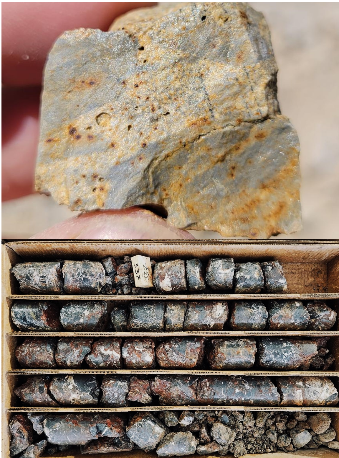
Photo 1. Diamond drill core rubble from hole RVD21-001 collared on the G1 gravity low target, interpreted to be a volcanic diatreme breccia pipe. Upper Photo: Ten metres from surface; fine (~1mm), deep red oxidized sulfide grains of pyrite/arsenopyrite disseminated in decalcified and clay altered limestone host and typical of Carlin-style gold mineralization. Lower Photo: from 103m to end of hole; chaotic, brick-red gossan-cemented angular breccia with mixed fragments of dark silicified carbonate and epithermal style quartz veins, indicative of a deep volcanic source.
