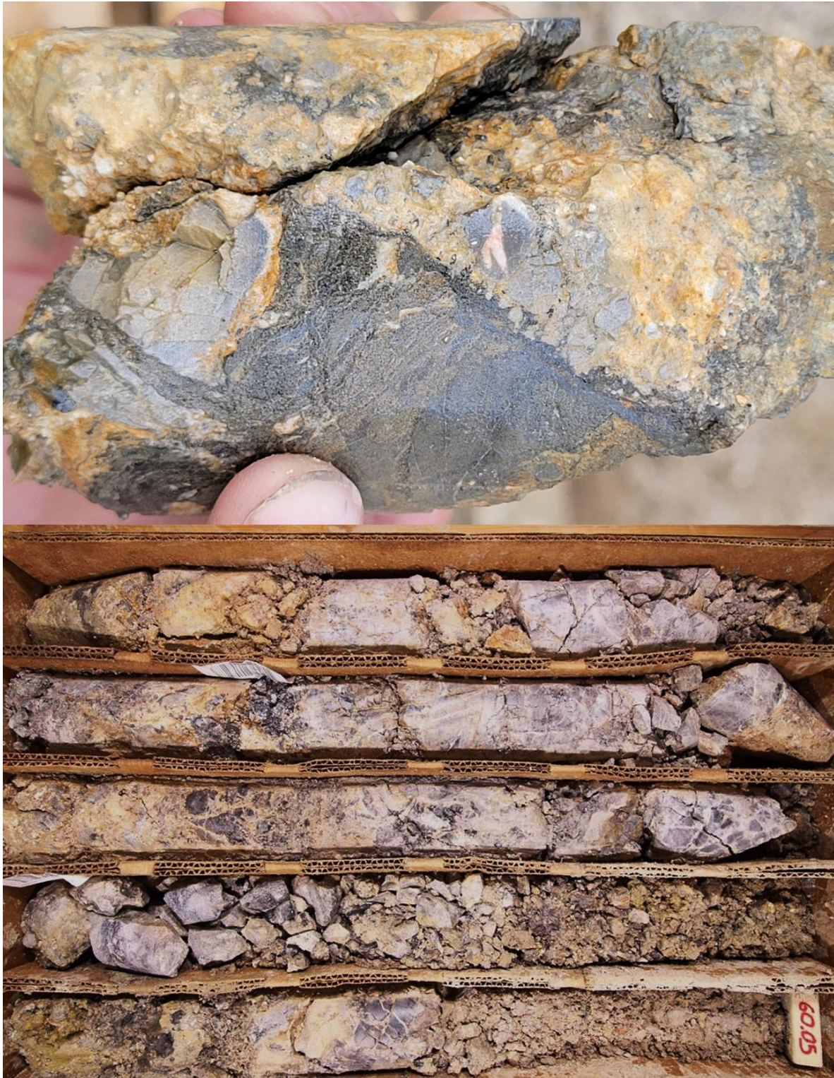
Photo 2. Drill core rubble from 60 m depth in hole RVD21-001 collared on the G1 gravity anomaly and breccia pipe target. Upper Photo: close-up photo of intensely clay - and silica-altered breccia with angular, dark grey silicified and lighter grey decalcified carbonate fragments with quartz-calcite veining in a clay rich orange gouge groundmass. Lower Photo: core box full of orange, iron-rich clay gouge holding together fragments of altered and silicified carbonate. The difficult drilling conditions encountered in G1 are the result of hydrothermal shattering during formation of the breccia pipe, and faulting.
